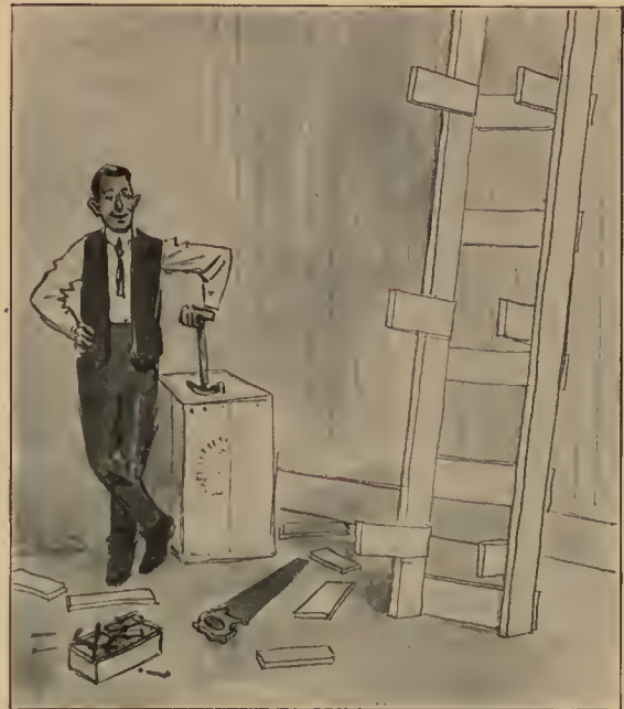
SHOWING HOW EASILY A RACK FOR STORING MOLDING ON END MAY BE CONSTRUCTED.
