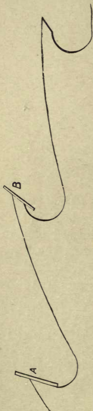
Fig. 13.—Testing for Need of Gumming.
