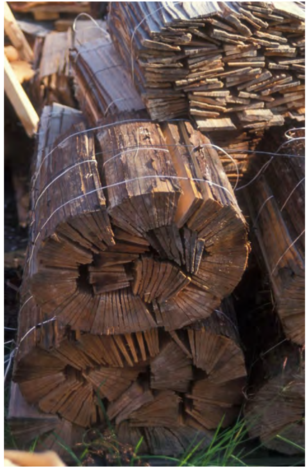
Figure 5.11 Cleaved shingles in one of the 'material banks' established as part of the programme to repair medieval timber structures in Norway 1991-1996.
