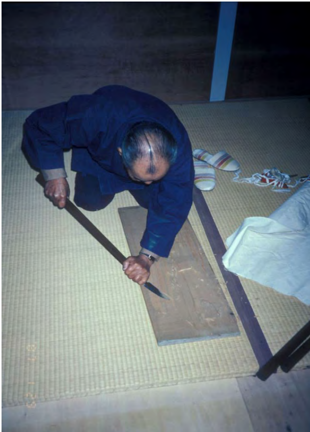
Figure 5.3 Tsunekazu Nishioka planing with the spear-shaped plane ( yari-ganna ). The Yakushi-ji Buddhist temple in Nara, Japan, 1987.
