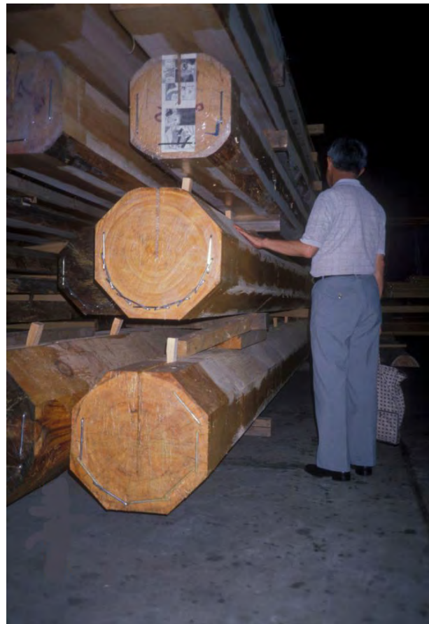
Figure 7.10 From a sawmill in Sakurai city, Nara, Japan. This sawmill specializes in Japanese cypress ( Chamaecyparis obtusa ). The ends of each log are waxed to stabilize the humidity inside the wood. Cramps are inserted into the ends to avoid cracking.
