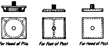
FIGS. 52f, g, and h. Cast-iron Bearing Caps.
